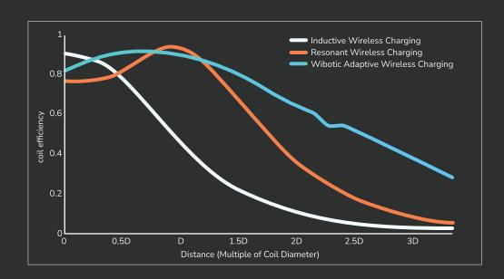
Adaptive wireless charging provides superior antenna range.
